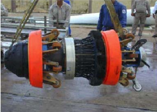
Figure 1: Geopig™ ready for launching.
